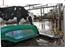
The new Joz robot scraper has been installed with its docking station where it recharges its batteries and takes on water for the system that sprays ahead of the scraper. It is doing a great job especially in the crucial area along the heel-stone. It is programmed to scrape the cubicle area eight times a day and the feed area twice a day. We have seen immediate benefits in cleaner cows.
